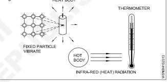
Transmission of heat takes place in three ways Conduction, Convection and Radiation.
