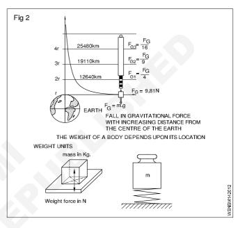
weight = W or FG = mass x gravitational force = m x g
