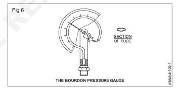
In I.C. Engines, Bourdon tube pressure gauges are widely employed for measurement of pressure, temperature and vacuum. In these gauges, a Bourdon tube which is a tempered, one is used and it attempts to straighten out under pressure and temperature and contact under vacuum.
