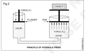
$\frac{\text{Force on plunger}(F)}{\text{Plunger area}(a)} = \frac{\text{Weight on the ram}(W)}{\text{Ram area}(A)}$
