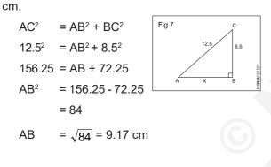
8 A ladder of 12.5 metre long is placed with upper end against a wall. The lower end being 7.5 metres from the wall. What height is the upper end above the ground.
