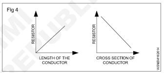
4 depends on the temperature of the conductor
