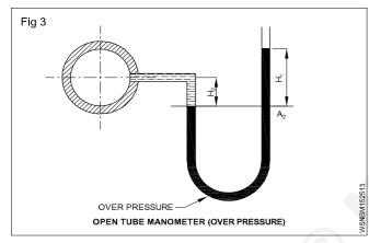
It is more suitable to measure pressure in vessels which is having little variation to atmospheric pressure. It is a 'u' shaped tube containing mercury having its one end connected to the vessel container in which the liquid is there whose pressure is to be determined. The other end is open. The manometer will show a difference in both the limbs of the tube when the pressure inside the vessel is more or less than the air pressure outside.
